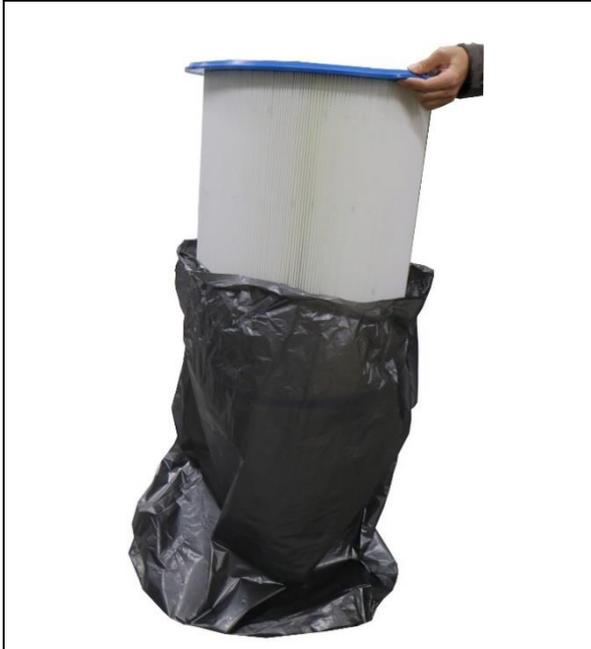
6.) Place the used filter element in the packaging provided for this purpose.
