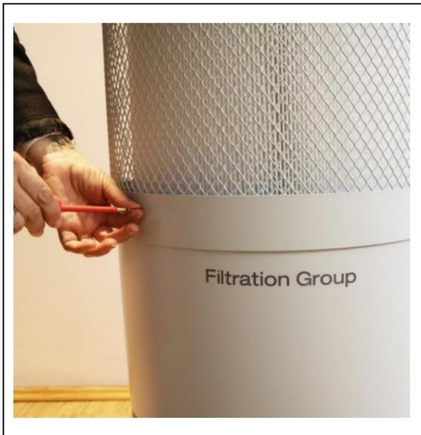
3.) Loosen the locking screws for the housing.
