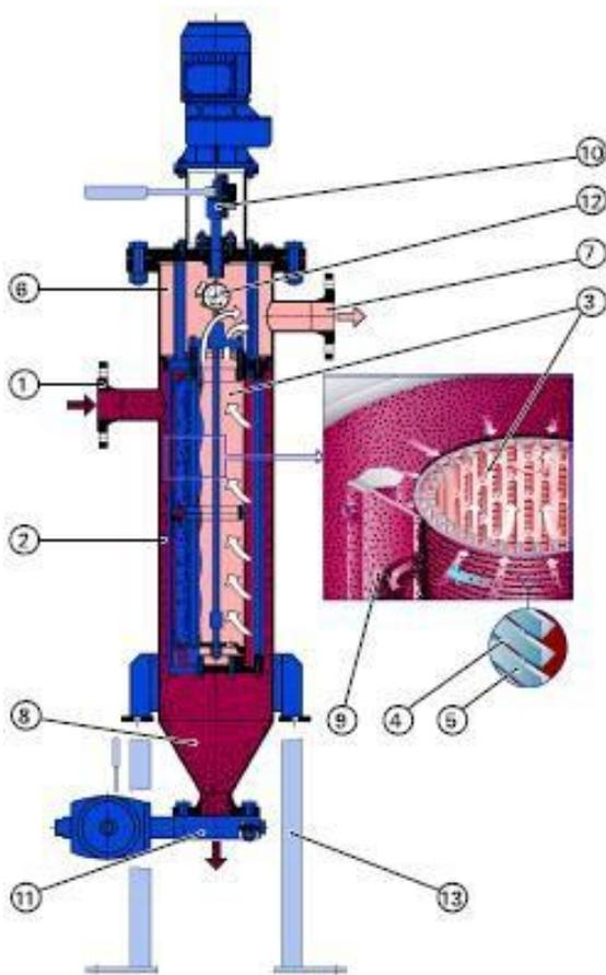
The filtered fluid exits the filter housing at the top opposite the inlet connection. In the AF 93 S version, the integrated preseparator relieves the filter cartridge of coarse and heavy particles by means of a tangential flow around the tube.
