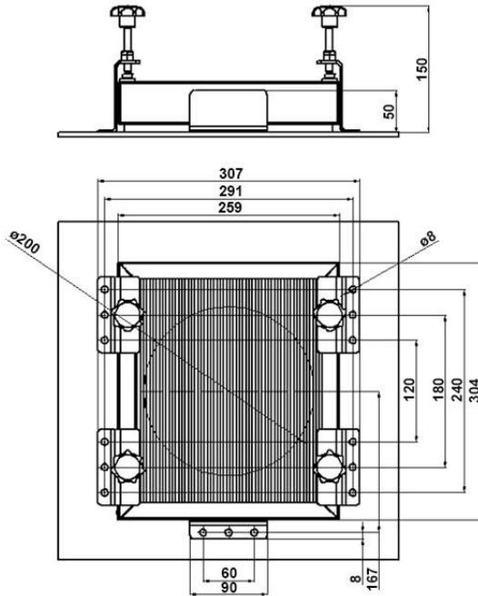
MIO filter plates are cleanable coarse filters that can reach filter class G4 (EN 779) depending on the inflow speed
