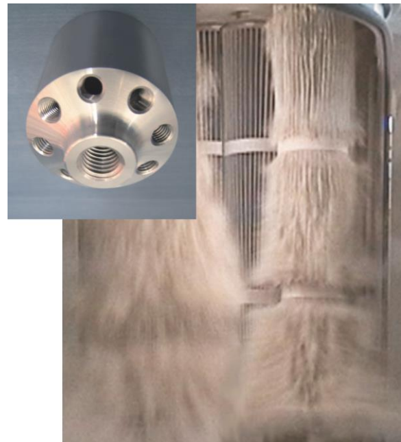
Cleaning by means of a multi-jet nozzle
